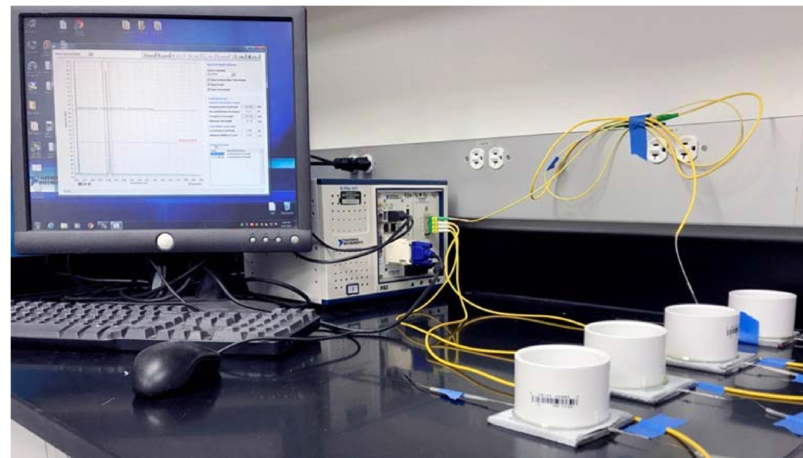
Figure 2. Accelerated corrosion test setup.
